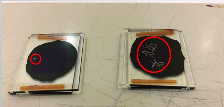
Image of broken samples during poling process.
